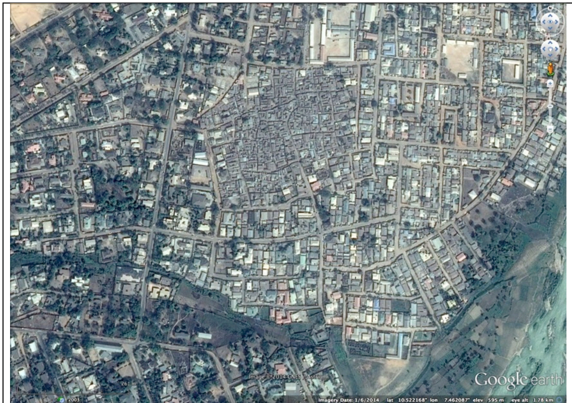
Kaduna – urban village (traditional, informal layout), lower middle income (50' x 100' lots – informal) and upper income (GRA – formal 100' x 100' lots) housing areas
