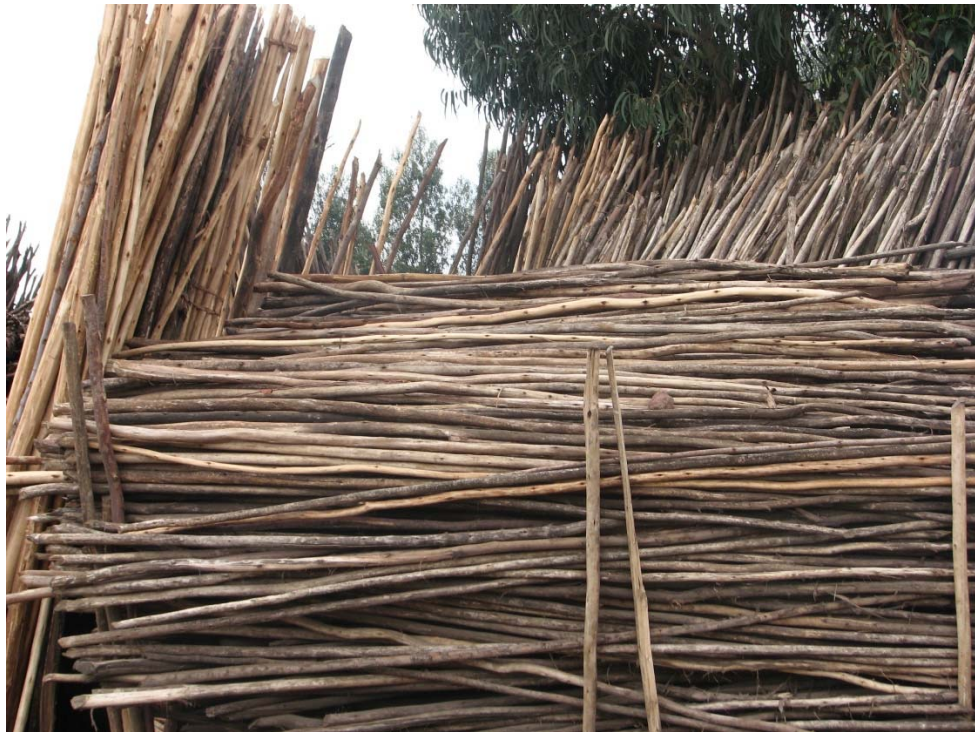
Picture 2 Eucalyptus poles for scaffolding, walls, and roof trusses
