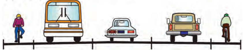
Figure 7.6. This road diet shows four lanes reduced to two lanes, a center turn lane, and two bike lanes.
