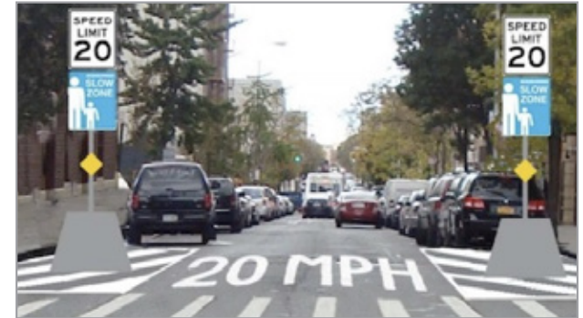
Figure 13. An Engineering Action like the Slow Zones, seen above, can help manage speeds in neighborhoods or areas with schools, senior centers, or other uses that draw vulnerable users. (Source: NYC Streetsblog)
