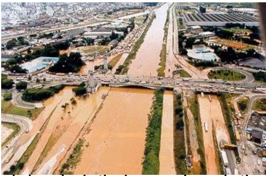
Floods due urbanization increase, river reduction capacity (solids and sediments), and occupation of the valley
