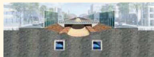
Stage 4: Sewer and bridge construction (September 2004)
