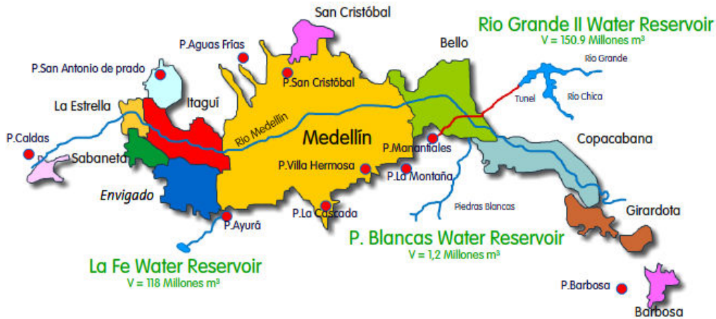
Figure 7.8 Water Supply “lay-out” for Metropolitan area of Medellín (red dots are the water treatment plants (source: EPM)
