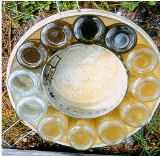
Figure 1.21 Samples of stormwater water quality distributed as a watch where the first sample is between 15 and 10 minutes before the hour. It can be seen by the colour shows how polluted is the water in the beginning of the hydrograph.
